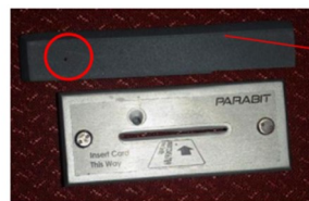
Door Access Device Skimmer & PIN Capturing Device
